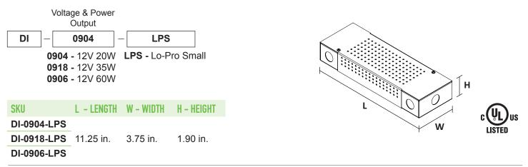
**LO-PRO**<sup>®</sup> JUNCTION BOX & DRIVER COMBO - 12V COMMERCIAL GRADE 0-10V LED DIMMABLE DRIVER Compatible with 0-10V controls and dimmer systems.
